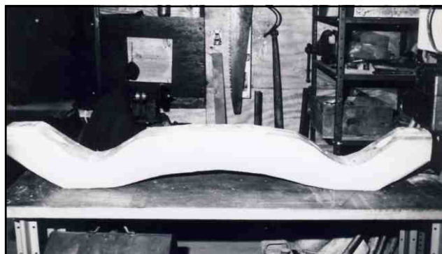
Picture 14. The yoke roughed out front and back, and top and bottom.
