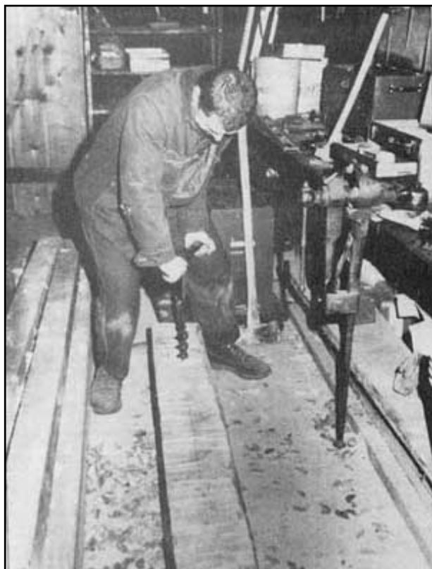
Pictures 8 and 9. Using the template in Diagram 3, draw the top lines and drill the holes.
