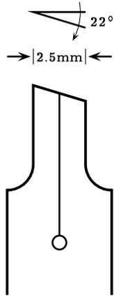
Pens with nibs pre-ground to the correct angle are not generally available, so start with an inexpensive calligraphy fountain pen (Schaeffer, Platignum, etc.) and file the end of the nib to 22° as shown. File across the nib (in the sketch, into the paper) and finally remove the sharp edges by ‘writing’ on 1000-grit water paper on a firm flat surface.
